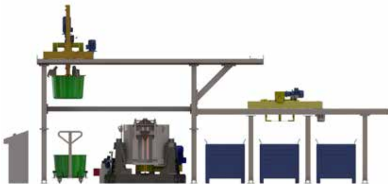
■ Configuration with three discharge stations. Detail: spun swarf discharge
